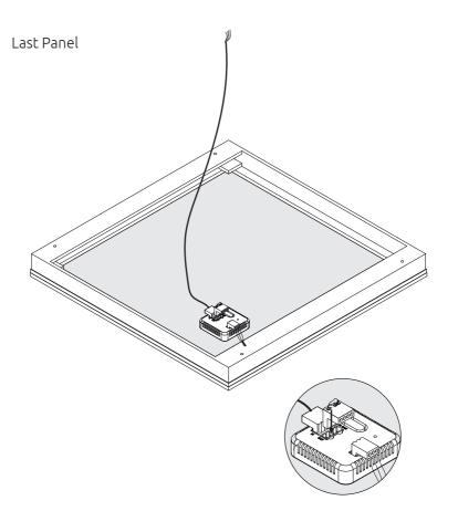
On the last panel in the series, you must place the supplied end terminal in the "Out" connection
